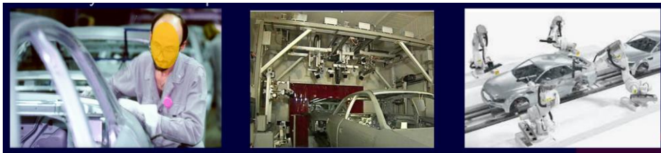
Figure 8: Evolution of the Automatic Body Inspection System “ABIS” from manual to robot-based
