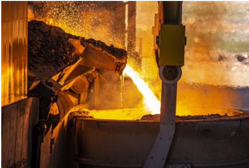
Figure 22: Molten metal transferred to the ladle before casting 27
